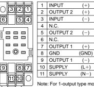
Note: For 1-output type models, the terminals for OUTPUT 2 are not connected.
