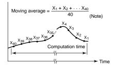
Note: For the moving-average times of 3, 2, and 1 second, the number of samplings is 30, 20, and 10, respectively (when the computation cycle is 100 ms). Setting range of moving-average time: 0 to 320000 seconds
